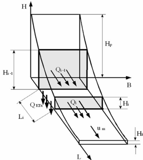
Fig. 3. Mass balance of particular sections of the screen
